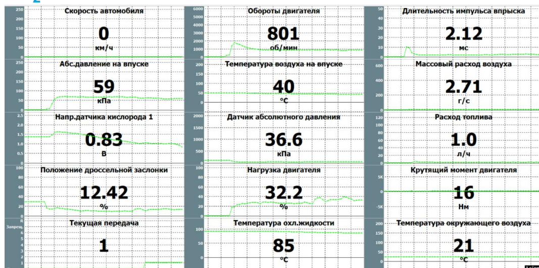
Figure 2. Software interface for collecting vehicle OBD II parameters.
