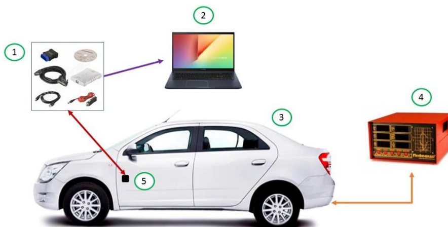
Figure 1. Connection of devices. 1 – scanmatic, 2 – computer, 3 – car, 4 – gas analyzer, 5 – place of connecting cable of scanmatic.
